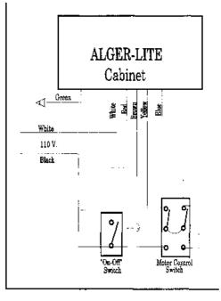
4. **ROUGH IN:** Run 5 ea. #14 Ga. wires from the place where the ALGER-LITE is mounted to the switches. **NOTE:** This must be done in accordance with local electrical codes. Connect wires as indicated in diagram on page 1. and fasten ALGER-LITE cabinet to cover with four machine screws.
